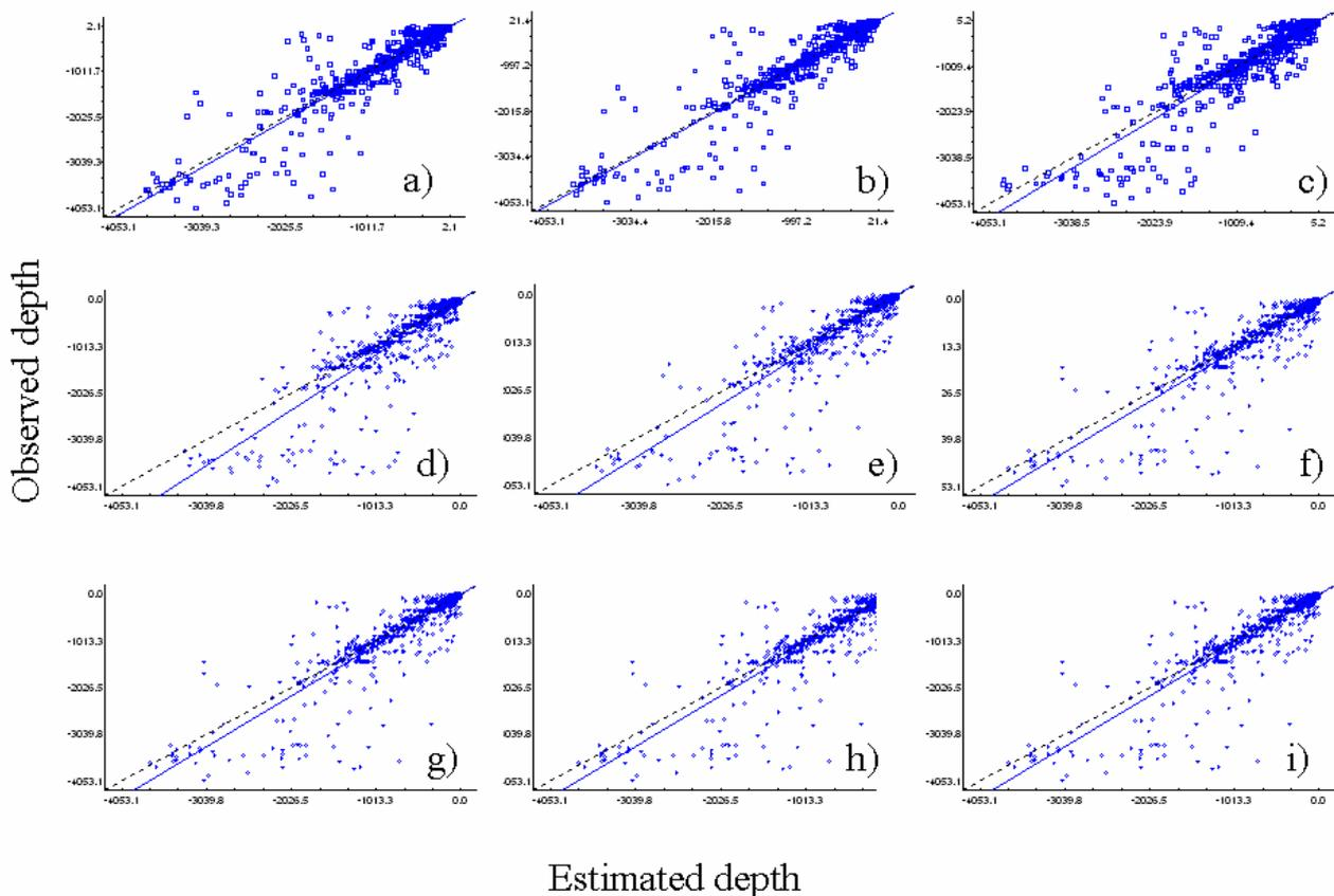
**Figure 4.** Results of cross validation analysis used to compare the interpolation methods: a) spherical kriging, b) exponential kriging, c) gaussian kriging, d) inverse distance-1, e) inverse distance-2, f) inverse distance-3, g) inverse distance-4, h) inverse distance-5, i) inverse distance-6 (Dotted lines represent a perfect fit 1:1).
