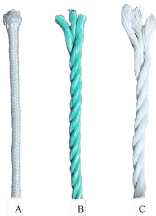
Figure 1. Detail of ropes used at the experimental phase: nylon (A), raffia (B) and polypropylene (C).
