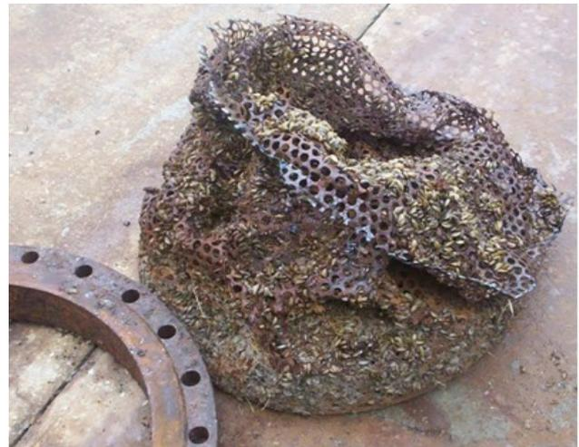
**Figure 2.** Macrofouling by *L. fortunei*. The photograph was taken in summer 2007; it shows a damaged part of the water pumping system at Laguna del Sauce after colonization by this invasive bivalve.
